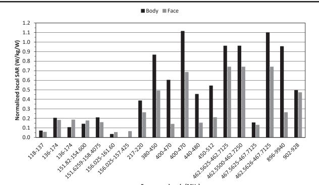
Figure 3 — Local ten-gram averaged SAR produced by commercial handhelds that operate near or within amateur radio bands (based on 50% PTT duty cycle and 1 watt).
